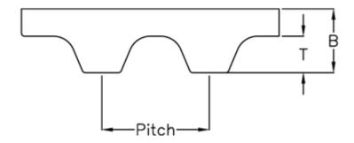
Height B mm= 2.2Height T mm= 1.2Length= 990Number of teeth= 198Pitch= 5Type $= PU \ 8 \ T5 \ 990$ Width= 8
